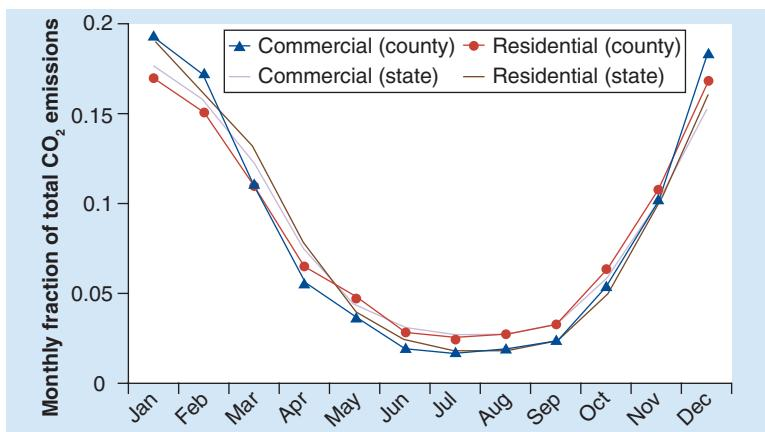
**Figure 7. Comparison of the monthly fractions of residential and commercial department of energy/energy information administration state-total natural gas consumption to the on-site residential and commercial fossil fuel CO<sub>2</sub> emissions estimated in this study for Marion County, Indianapolis, USA.**
