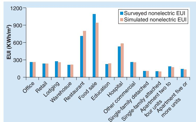
**Figure 3. Comparison of simulated (after calibration) and surveyed nonelectric EUIs for commercial and residential buildings.** The two age cohorts have been combined for all buildings.
