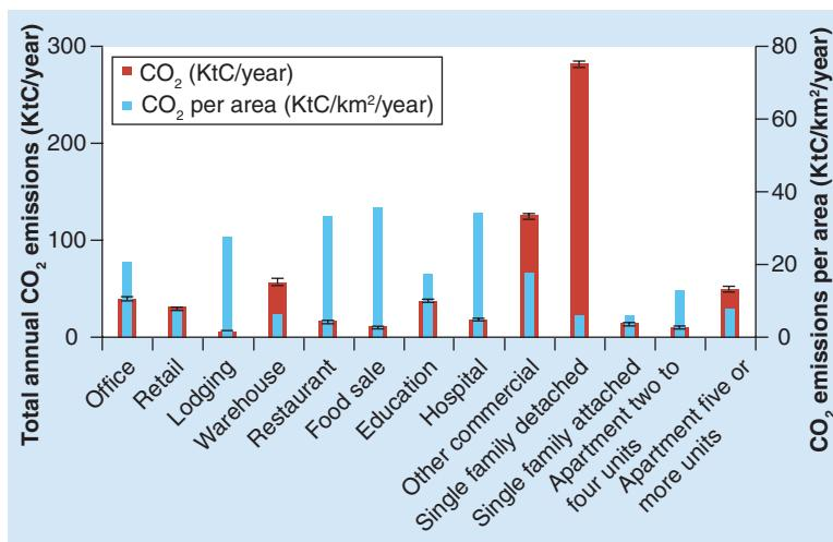
**Figure 9.** Annual total commercial and residential on-site fossil fuel  $\text{CO}_2$  emissions (with 95% confidence interval) summed by building category and the emissions per unit area.
